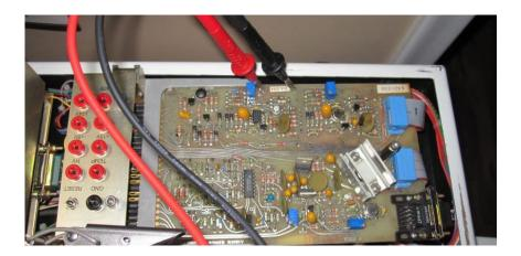
In the next picture the shutter motor circuit is turned on constantly by connecting a ground (green wire) to control line at anode of diode D302. To adjust the setting the potentiometer R314 is adjusted while monitoring voltage across R301. Typical results are shown above. The run-stop test is used to test if final settings are optimal.
